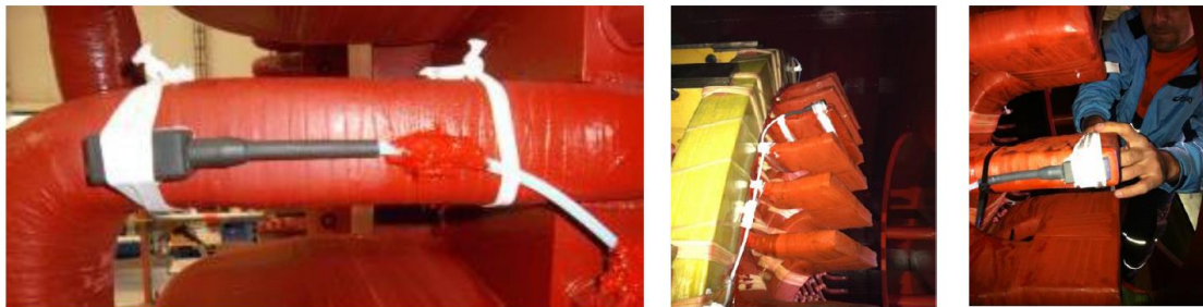
Figure 3: Example of a Fibreoptic Accelerometer Sensor
